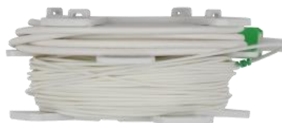
Side view of the EZ Connect two-layer spool assembly. The lower layer includes the 900 \mu m micro-drop. The upper layer includes the shorter-length jumper layer that will be plugged into the ONT.
